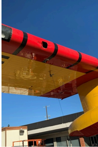
Drone Collision Damage
