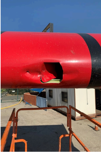
Drone Collision Damage
