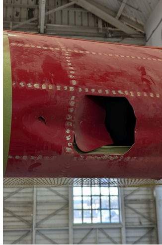
Drone Collision Damage
